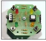
Before you put any components in the board or pick up the soldering iron, just take a look at the Printed Circuit Board (PCB). The components go in the side with the writing on and the solder goes on the side with the tracks and silver pads.
