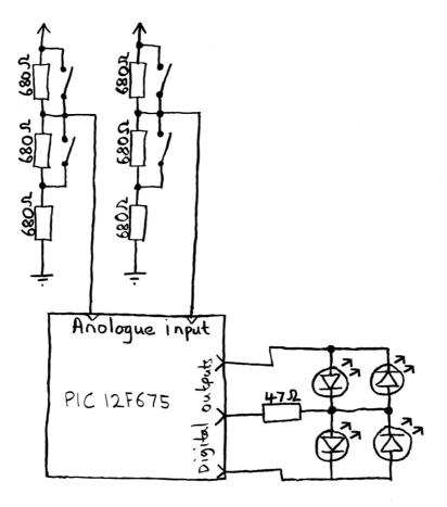
At the heart of the electronic circuit is a microcontroller. A microcontroller is in effect a small computer. The circuit uses a cleaver design to allow four switches and four LED's to be connected to only five input / outputs.
